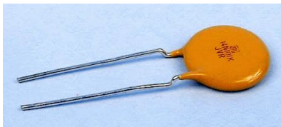
VDR Voltage Dependent Resistor
