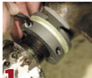
1 Coming in two parts or more, a scissor cutter can be attached without removing the prop
