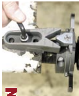
3 The fixed cutter is held in place by this block, which must be tapped into the P-bracket
