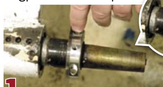
1 Solid discs will require the prop to be removed
