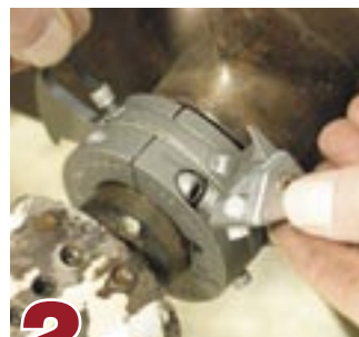
2 The fixed blade fitted here sits on a bearing which will have to be replaced every two years or so
